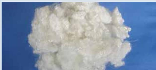
3. The plastic chips are melted down and then extruded into a new fiber.
