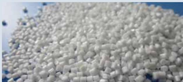
2. PET bottles are sterilized, dried and crushed into small chips.
